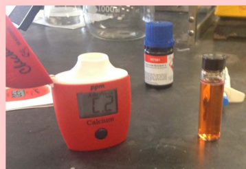
Right: An image of calcium levels being tested utilizing the Hanna H1758 Marine Calcium Tester
